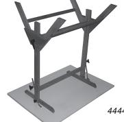
Before securing base of table to Drawing Board top, you must center the base to the top.
