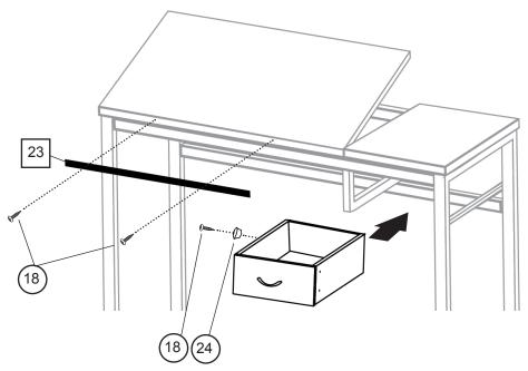
Attach pencil ledge (Part 23 ) to the front edge of table top, using two 4x12mm screws (Part 18).
