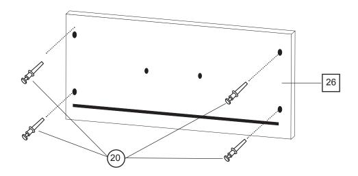
C) Take the drawer front panel (Part | 26 ) and insert 4 threaded composite bolts (Part (20) ). Use Phillips head screwdriver to secure threaded connector pins.
