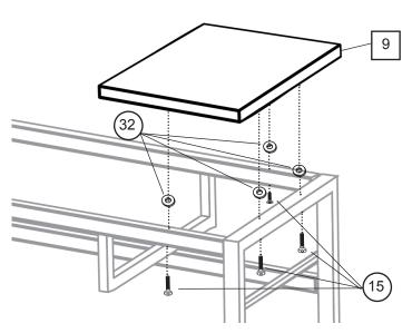
Line up the drawer top (Part 9 ) to the specified holes on table base. Once drawer top is positioned correctly, secure top using 4 of 6x28mm bolts (Part 15) and 4 of the metal washers (Part 32). The metal washers should be positioned between drawer top and table base.
