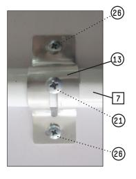
Now place the Board Brace Clamps (Part (13)) over the Board Brace (Part (7)) on the backside of the Table Top (Part (1)) and line up the Board Brace (Part (7)) with two of the pre drilled holes.
