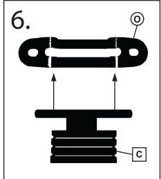
Attach backrest plate ① to backrest support bar C by inserting backrest support bar H into longated slot in backrest plate ① . Continue with Step 7
