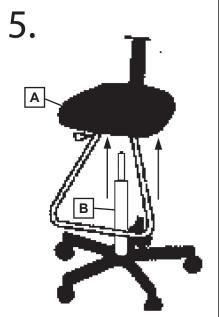
Take the complete seat assembly and insert the seat plate of the cylinder  $\boxed{\mathsf{B}}$  by inserting the cylinder into the hole on the bottom of the seat plate  $\boxed{\mathsf{A}}$ .
