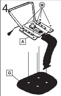
With seat cushion lying plastic side up, line up [4] holes in seat plate A with [4] holes in Seat Cushion G. Attach with [4] 5/8" black bolts M. Tighten securely. Please note: Foot bar should face front of seat cushion (Front of cushion has label attached.)
