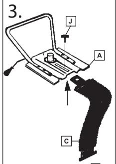
Attach Backrest Support Bar C to seat plate A by sliding the bar into the raised area of the seat plate (see arrow for location).
