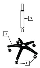
Place base D face down and push castors E in firmly. Insert cylinders
