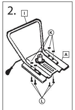
Attach foot bar I to base plate A using [4] 1 1/4" Bolts L and [4] nuts K. Line up holes in footbar to holes in seat plate. Tighten Securely.
